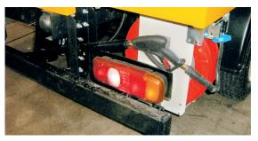
High-pressure washer 15l/100 bar with automatic drum and spay lance
