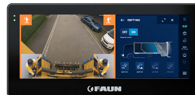
Standard equipment: Work area monitoring in accordance with EN 1501-1:2021, displayed as "picture-in-picture" on 7"
