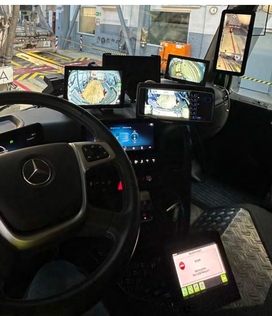
Situation in the cab: Separate displays from different providers lead to a confusing display and operating environment.
