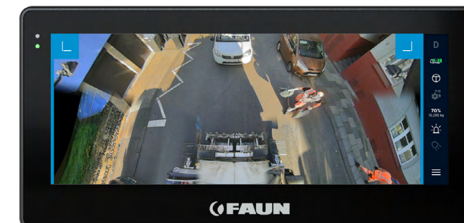
Optional: Work area monitoring in accordance with EN 1501-1:2021, displayed as a "digital rear-view mirror" in full-screen format on 12"
